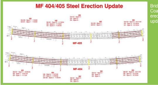
Bridges over Coal Valley Road erection framing update.
